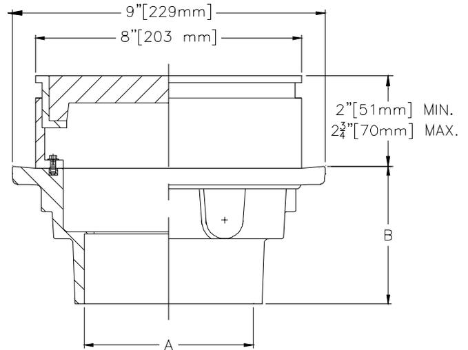
**FD-2330 Heavy-Duty Adjustable Floor Drain**
