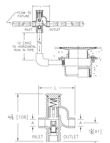
**Note:** Trap primer should be installed a minimum of 6" above grid of floor drain or flood level rim of equipment served.
