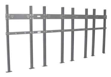
Multiple station plate system provides an extended length plate fabricated with exact center-to-center locations to accommodate a bank of multiple urinals. Custom-length plates are specific to job requirements and are provided with loose uprights and boxed mounting hardware and studs. Ideally suited for prefabricated applications.
