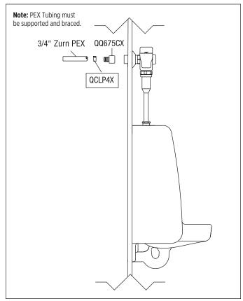
Urinal Flush Valve Operating (0.5 gpf or Less) Connection Example
