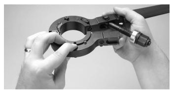
**Step 2:** Continue to hold in the keyed slot, turn tool around and move key out of position. Remove jaw from clamp.
