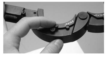
Step 3: Insert new crimping jaw.
