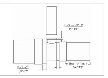
This spacing generally ensures the crimp ring is centered over the ribs of the fitting. For worry-free spacing, the QickCap Crimp Ring with positioning stop can be used to virtually eliminate ring movement during installation.
