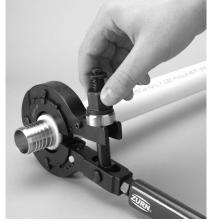
**Step 5:** Drive the nut down with an impact wrench until blue LED light turns on.
