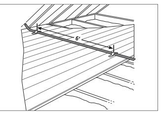
Straps can be 6 feet apart if the tube is continuously supported.
