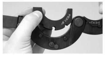
**Step 4:** Rotate key back into position until key clicks to lock jaw in place. Repeat for other jaw.
