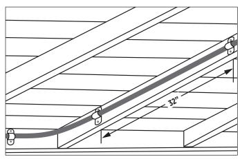
Straps can be 32 inches apart maximum in a horizontal run.
