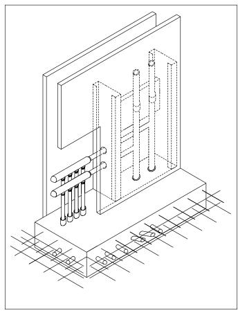
Example of Fixture Supply in Commercial Construction
