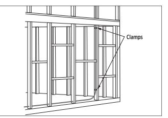
Vertical runs need supported on every floor. Depending upon the type of construction method being utilized, mid-story guides may be required (see section on Commercial Construction Methods).
