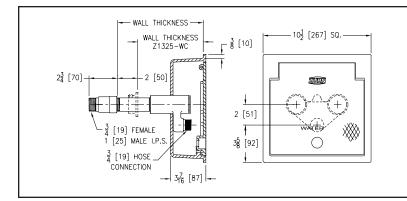
ENGINEERING SPECIFICATION: ZURN Z1325 "Vari-Temp" combination hot and cold water, nonfreeze, encased wall hydrant for flush installation. Complete with bronze casing, all bronze interior parts, non-turning operating rods with free-floating compression closure valves, replaceable bronze seat and seat washer, and combination 3/4" [19 mm] female or 1" [25 mm] male straight IP inlet. Nickel bronze box and hinged cover with operating key lock and "WATER" cast on cover.
