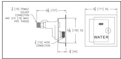
**ENGINEERING SPECIFICATION:** ZURN Z1330 Encased Ecolotrol anti-siphon wall hydrant for moderate climate and interior wall installation. Complete with integral backflow preventer, all bronze interior parts, with one-half turn ceramic disc cartridge and combination 3/4" [19 mm] female solder and 3/4" [19 mm] male pipe thread inlet. Stainless steel box and hinged cover with operating key lock and "WATER" stamped on cover.
