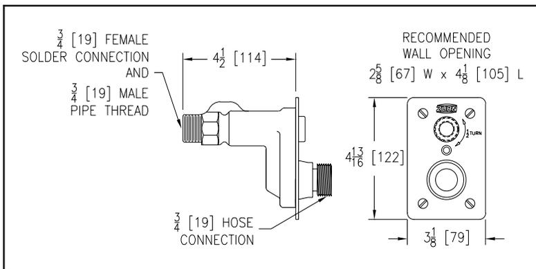
**ENGINEERING SPECIFICATION:** ZURN Z1333 Exposed Ecolotrol anti-siphon wall hydrant for moderate climate and interior wall installation. Complete with integral backflow preventer, all bronze interior parts, with one-half turn ceramic disc cartridge and combination 3/4" [19 mm] female solder and 3/4" [19 mm] male pipe thread inlet. Stainless steel face with operating key.
