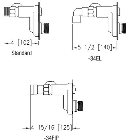
**Z1333 ECOLOTROL WALL HYDRANT WITH CERAMIC DISC** Parts Assembly and Parts List
