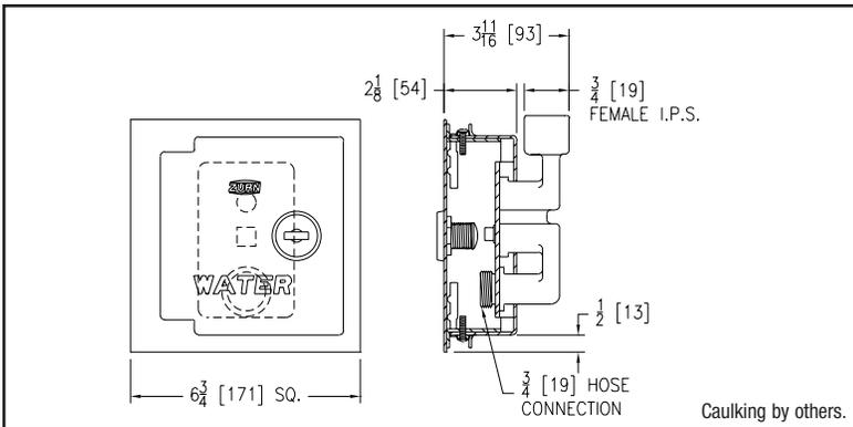
**ENGINEERING SPECIFICATION:** ZURN Z1350 Encased moderate climate wall hydrant for narrow wall installation. Complete with bronze body, all bronze interior parts, replaceable seat washer, screwdriver operated stop valve in supply, key operated control valve, and 3/4" [19 mm] IP female inlet and 3/4" [19 mm] male hose connection standard. Stainless steel box and hinged cover with cylinder lock and "WATER" stamped on cover. **Note:** Caulking of inside joints by others.
