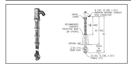
**ENGINEERING SPECIFICATION:** ZURN Z1390 Exposed, non-freeze post hydrant. Complete with bronze casing and cast aluminum casing guard, all bronze interior parts, bronze seat and replaceable seat washer, and non-turning operating rod with free-floating compression closure valve with 1-1/4" [32 mm], 1-1/2" [38 mm], or 2" [51 mm] connection. "T" handle operating key included. Hydrant is equipped with a tapped 1/4" [19 mm] drain port in valve housing.
