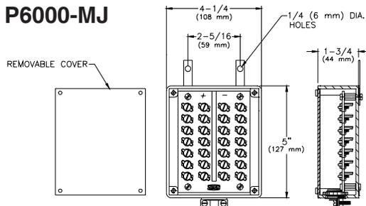
**ENGINEERING SPECIFICATION: Zurn P6000-MJ** - The Mini Junction Box is a 4-1/4" [108mm] x 5" [127mm] x 1-3/4" [44mm] electrical enclosure designed to connect up to ten Zurn sensor urinals/closets. The unit includes a high impact plastic enclosure with polarity marked terminal board, high impact plastic cover panel, wall mounting tabs, integral strain relief, and illustrative wiring diagram.
