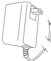
**ENGINEERING SPECIFICATION: Z6000-PC6 Plug-In Power Converter** - Plug-in Power Converter is designed to provide 6VDC power for 1-10 Zurn 6VDC sensor flush valves. Power converter plugs into 120VAC outlet (supplied by others) located convenient to flush valves. Electrical characteristics: Input: 120VAC 60Hz 35w Output: 6VDC 1.5A
