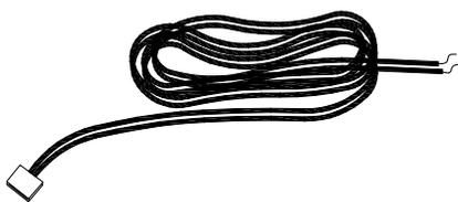
**ENGINEERING SPECIFICATION: Zurn PEMS6000-CW-IS Connecting Wire** - Connecting wire for ZEMS-IS to connect power to sensor operator. Comes with molex connector and is 10' in length. Wire is 24 gage.
