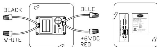
**ENGINEERING SPECIFICATION: Zurn P6000-HW6 Hardwire Power Converter** - Hardwire power converter to power up to 10 Zurn sensor urinal/closet flush valves or up to 8 hardwired Zurn sensor faucets. The P6000-HW6 is mounted on a 4-11/16" x 4-11/16" cover plate that mounts to a standard 4-11/16" x 4-11/16" electrical box (supplied by others).
