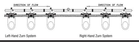
Stand facing the fixture. If flow is from the right, Zurn System is right-hand. If flow is from the left, Zurn System is left-hand.
