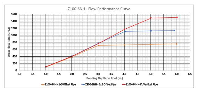
Example: The flow curve below shows that a 6-in. outlet drain with a 2-ft. x 5-ft. pipe configuration, and a ponding depth of 2.0 inches will yield a drain flow of 405 GPM.
