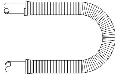
Step 4: Form the bend to the appropriate radius. A slight over bend initially helps the spring slide through after the final bend is formed.
