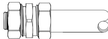
**Warning: When installing solder fittings, excessive heat may damage o-rings and isolators.**
