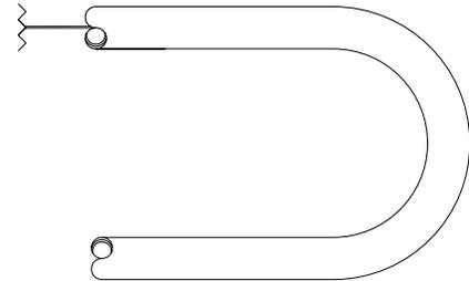
Step 5: Form the bend to the appropriate radius. A slight over bend initially helps the spring slide through after the final bend is formed.
