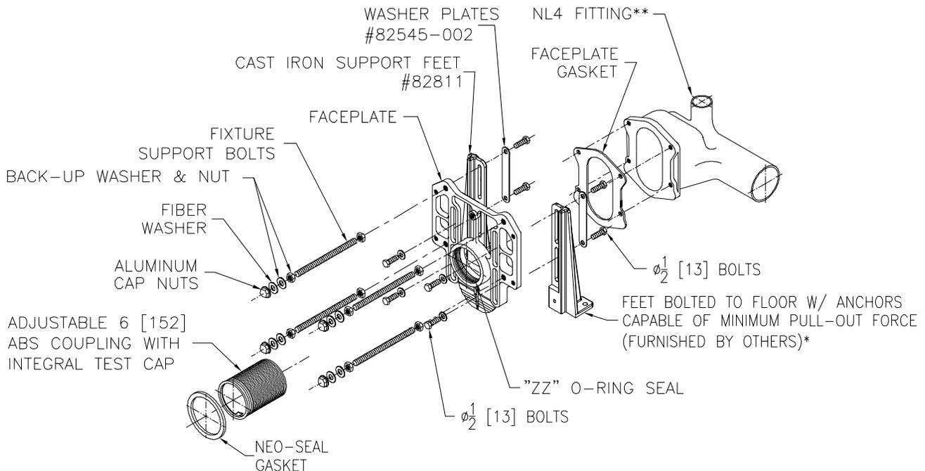
\*Carrier foot anchors must be able to withstand a pull-out force of 1004 Lb.[455 kg.]. Calculated value, no safety factor applied.
