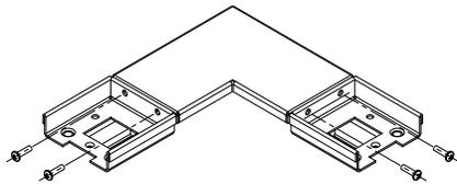
**STEP 11:** Install and secure the connector to the adjacent channel frames.
