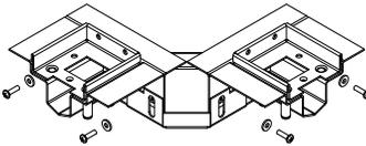
**STEP 3:** Install the washers and screws into the channel end caps.
