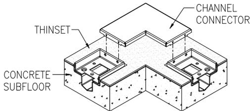
**STEP 10:** Apply thinset to underside of the channel connector.
