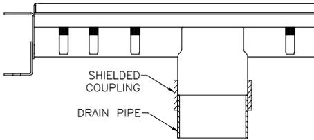
**STEP 6:** Attach the channel outlet to the drain pipe.
