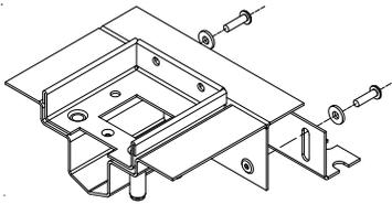
**STEP 1:** Remove the preassembled anchoring legs at the ends of channels that are being connected.
