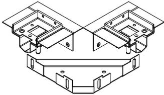
**STEP 2:** Install the connecting anchoring leg.
