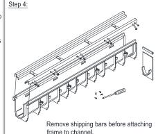
Perma-Trench offers a Heavy Duty (HD) frame option for intense traffic patterns. Simply slide the HD frame over the trench sections as shown below and attach with the hardware provided. Make certain that the notched end of the frame is at the male end of each trench section.
