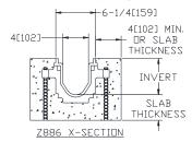
Specifying engineer is responsible for concrete encasement and reinforcing based upon application and local codes, as this may vary.
