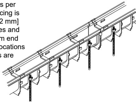
Typically, a trench system is assembled from the outlet on back. Starting with the deepest section or catch basin, set the first channel utilizing Perma-Trench's unique anchoring system. Integral rebar clips are located along the length of each trench drain and catch basin for easy attachment to #4 rebar stakes. Simply align the rebar stakes with the trench drain and drive them into the ground for positive anchoring. Attach the trench drain to the rebar stakes with the hardware provided.
