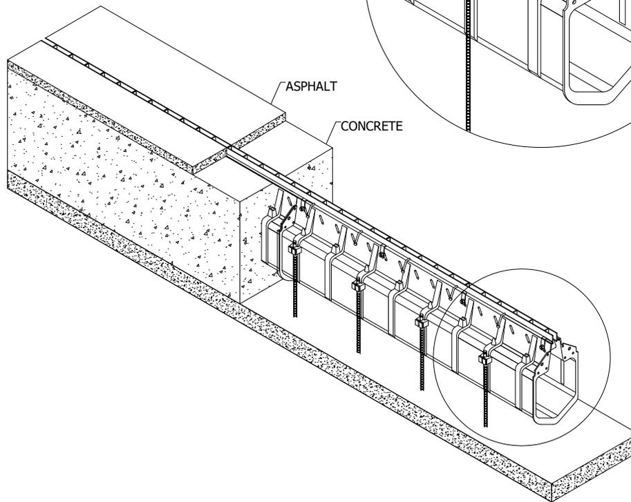
Our system can be installed with asphalt when using our special steel riser. It comes in two standard heights: 2" [50.8 mm] and 4" [101.6 mm]. Different heights are available upon request. The standard concrete installation is suggested around the Hi-Cap body for strength. A standard installation of the asphalt can be done up to a steel frame.
