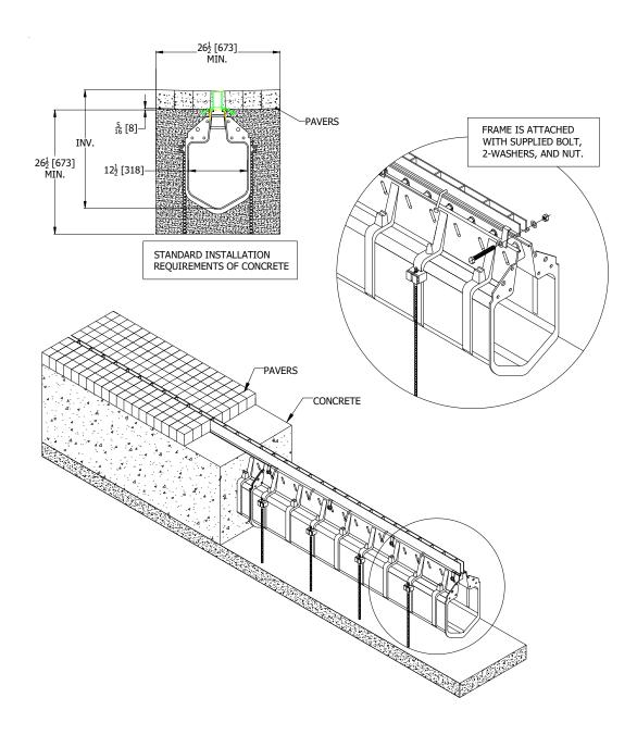
Our system can be installed with paving stones when using our special steel riser. It comes in two standard heights: 2" [50.8 mm] and 4" [101.6 mm]. Different heights are available upon request. The standard concrete installation is suggested around the Hi-Cap body for strength. A standard installation of the paving stones can be done up to a steel frame.
