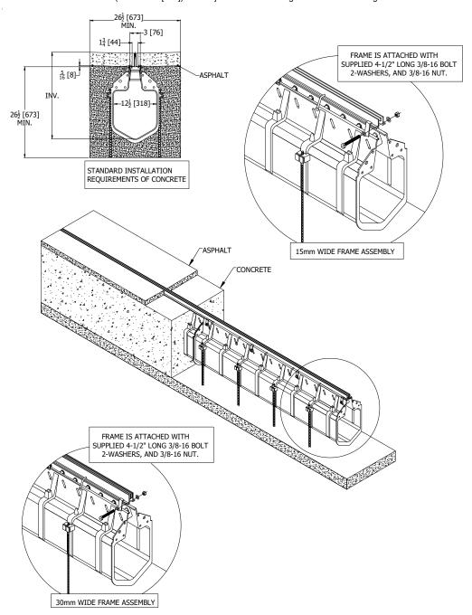
Our system can be installed with asphalt when using our heelproof frame. It comes in two standard heights: 50mm and 100mm and two standard widths: 15mm and 30mm. Different heights are available upon request. The standard concrete installation is suggested around the Hi-Cap body for strength. A standard installation of the asphalt can be done up to a steel frame.
