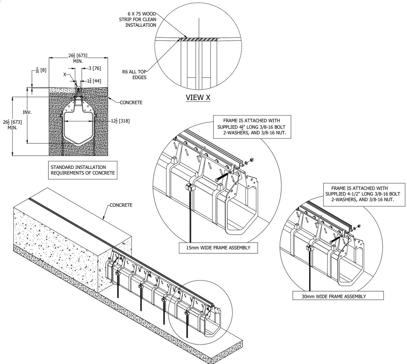
Our system can be installed with concrete when using our special steel riser. It comes in two standard heights: 50.8 mm and 101.6 mm and two standard widths: 15mm and 30mm. Different heights are available upon request. The standard concrete installation is suggested around the Hi-Cap body for strength. A standard installation of the concrete can be done up to a steel frame.
