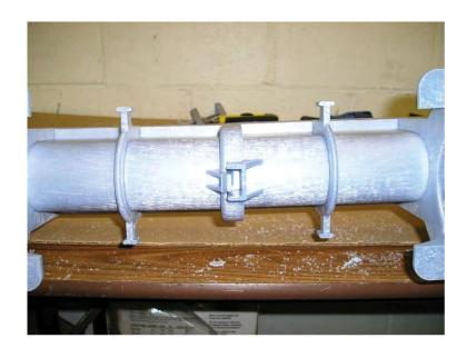
Assembling the trench run is easy using 'Flo-Thru's' mechanical interlocking joints. Simply align the male end above the female end and slide together. The bottom interlock should snap together. A silicone caulk, or a construction adhesive, such as Liquid Nails, is recommended to be used at each joint as a sealer.
