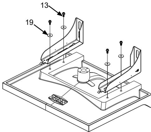
For ease of installation, lay basin on its top surface on a cushioned surface.
