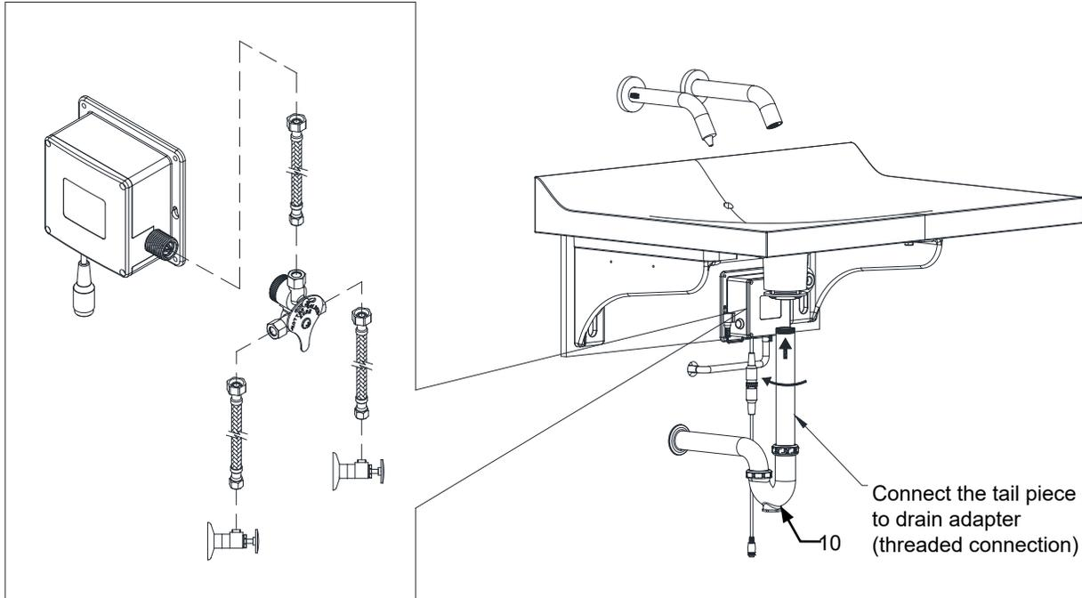
Adjust the tail piece base on drain outlet on the wall.
