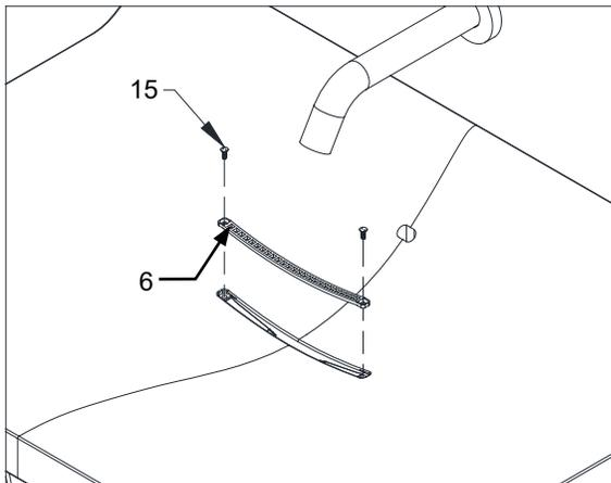
Use T10 Torx wrench to attach the grid drain to basin. Torque screws until the screw heads are flushed with the screw pocket of grid drain.
