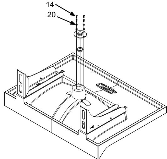
For ease of installation, lay basin on its top surface on a cushioned surface.
