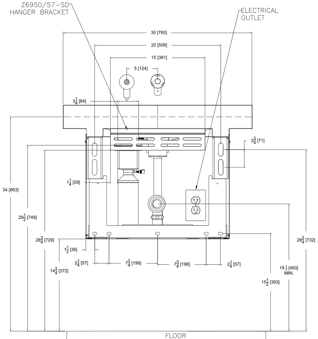
**Note:** Installing the P-trap outlet lower than 19.5" from finished floor will prevent the vandal shroud from being installed.
