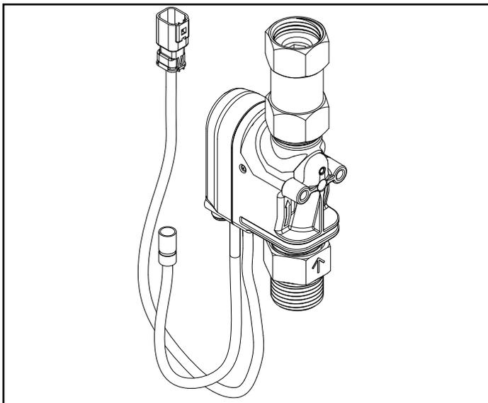
2.2. Tighten electronics module assembly to shank and connect water line(s).
