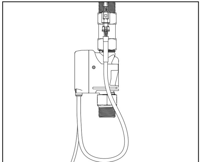
2.3a. Optional ACA version: Connect supplied inline connector and AC adapter.
