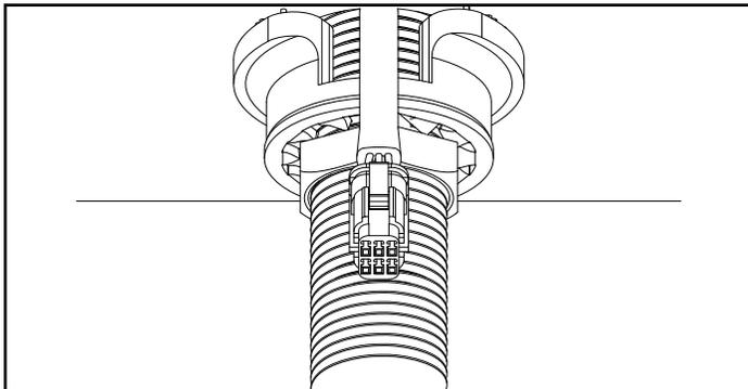
**!** Take care passing sensor cable through hole. Cable passes through front of plastic mounting washer
