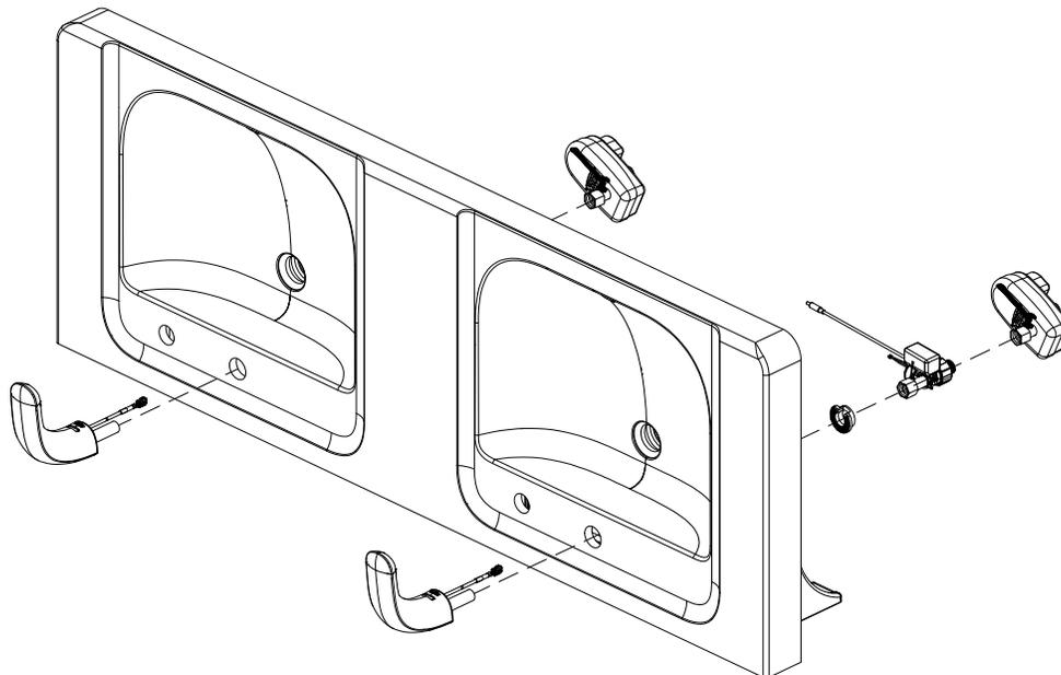
For ease of installation, lay basin on its back.
