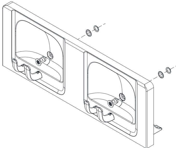
For ease of installation, lay basin on its back.
