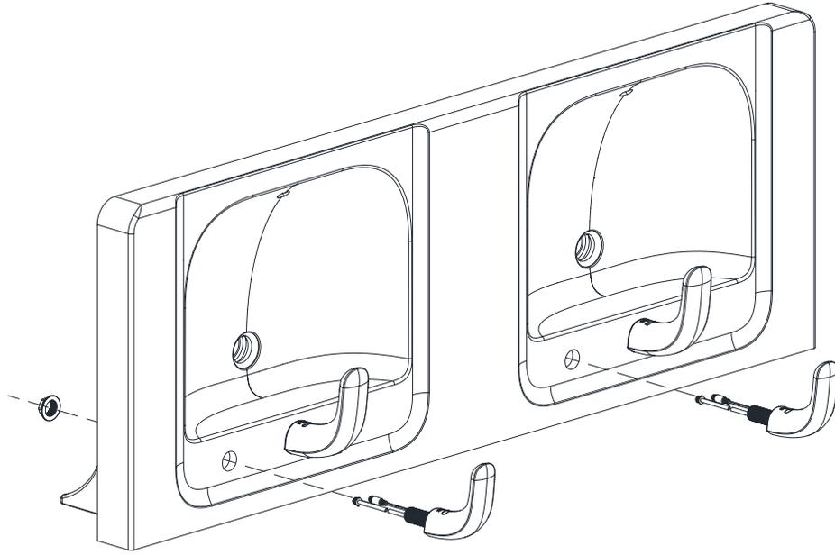
For ease of installation, lay basin on its back.
