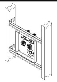
Step 3: Remove the paper backing from the gasket strip provided and adhere to the outer surface of the frame. Start from the top surface of the frame and wrap the gasket all around the frame. Make sure that the gasket is placed so that it is adjacent to the back corner of the frame cover (as shown in picture). Press firmly against the gasket to ensure that it makes sufficient adhesion with the frame.
