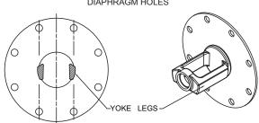
NOTE: Line up diaphragm screw holes with holes in body. Move yoke up and down checking for yoke contacting or dragging on valve body.
