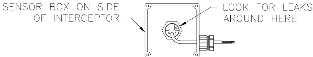
10. Replace cover on the interceptor and enclosure cover of the sensor box. If all steps were completed to this point, turn the power on.
