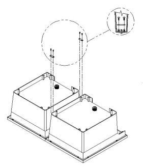
Attach the plastic connector to the four towel bar lugs on the underside of the sinks using the four screws provided.
