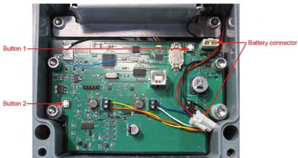
Control box with back cover removed
