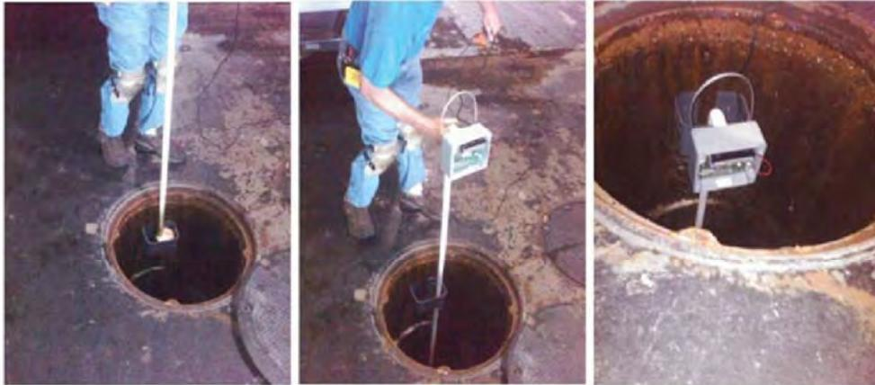
Remove cover from back of control box with 4 screws. Place probe through U-bracket and into interceptor until control box elbow rests on bracket (this is actually inserting the probe backwards at this point).
