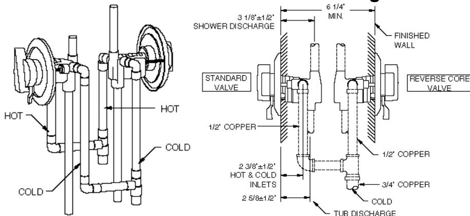
The ZURN TEMP-GARD Pressure Balancing Shower Valve is equipped with an adjustable limit stop screw. The limit stop device is to be used to limit the valve handle from being turned to undesired hot water discharge temperatures. To adjust the limit stop screw, remove handle and escutcheon, turn valve to maximum desired temperature and turn the limit stop screw until it seats.
