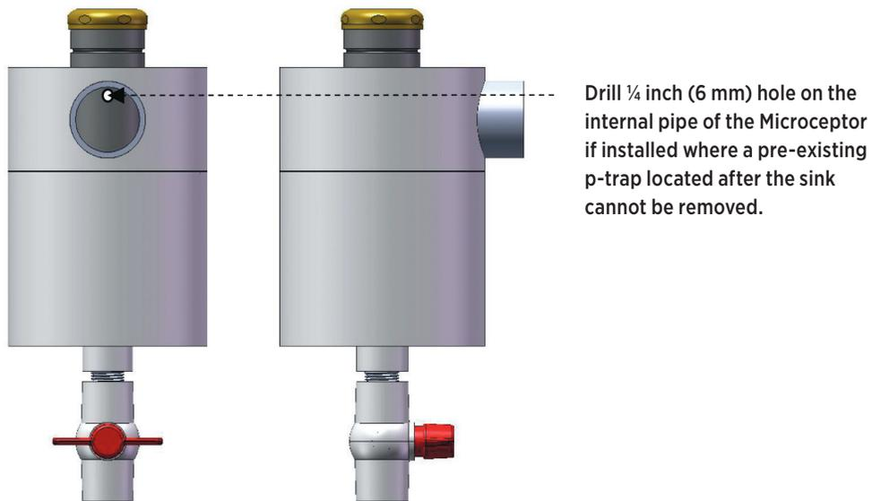
Figure 3 : For Retrofit Installations where pre-existing p-trap located after the sink cannot be removed.
