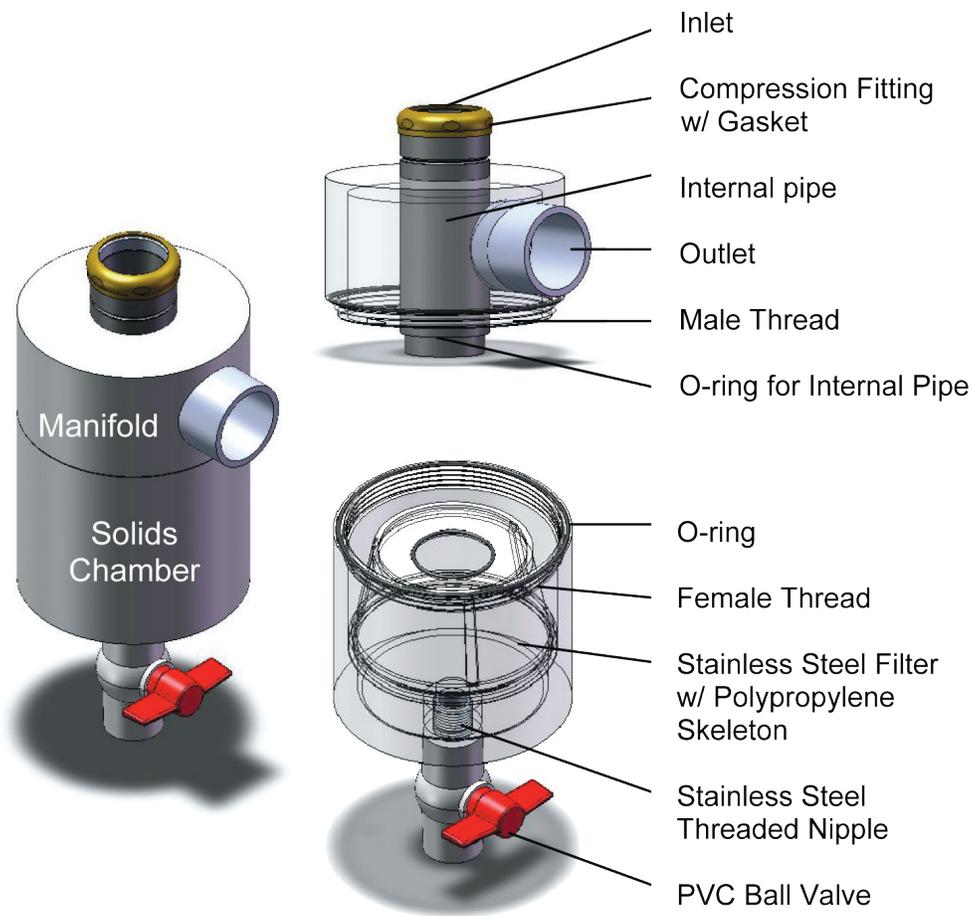
Figure 1: Microceptor Components
