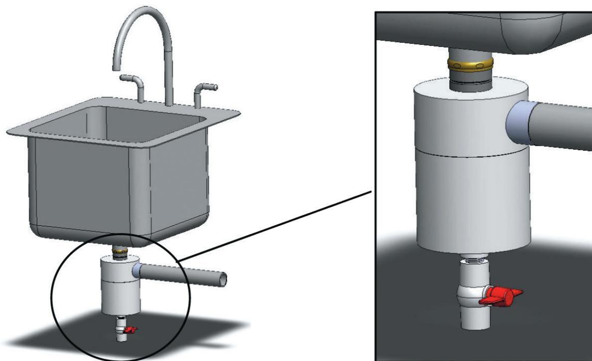
Figure 2 : Microceptor Installed Under Sink
