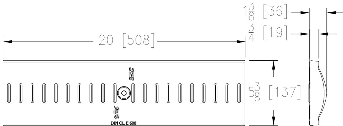
**DCE-USA GRATE ENGINEERING SPECIFICATION: ZURN P6-DCE-USA**
