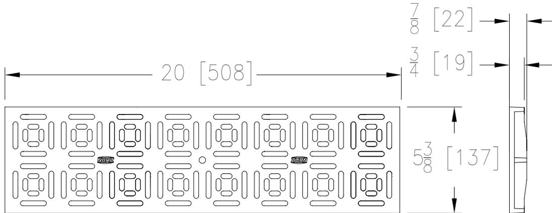
**NBZ-USA GRATE ENGINEERING SPECIFICATION: ZURN P6-NBZ-USA**
