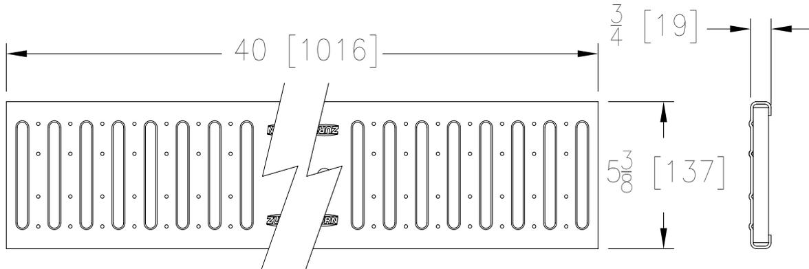
**FG GRATE ENGINEERING SPECIFICATION: ZURN P6-FG**
