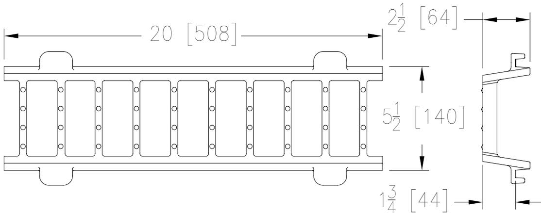
**HDD GRATE ENGINEERING SPECIFICATION: ZURN P886-HDD**
