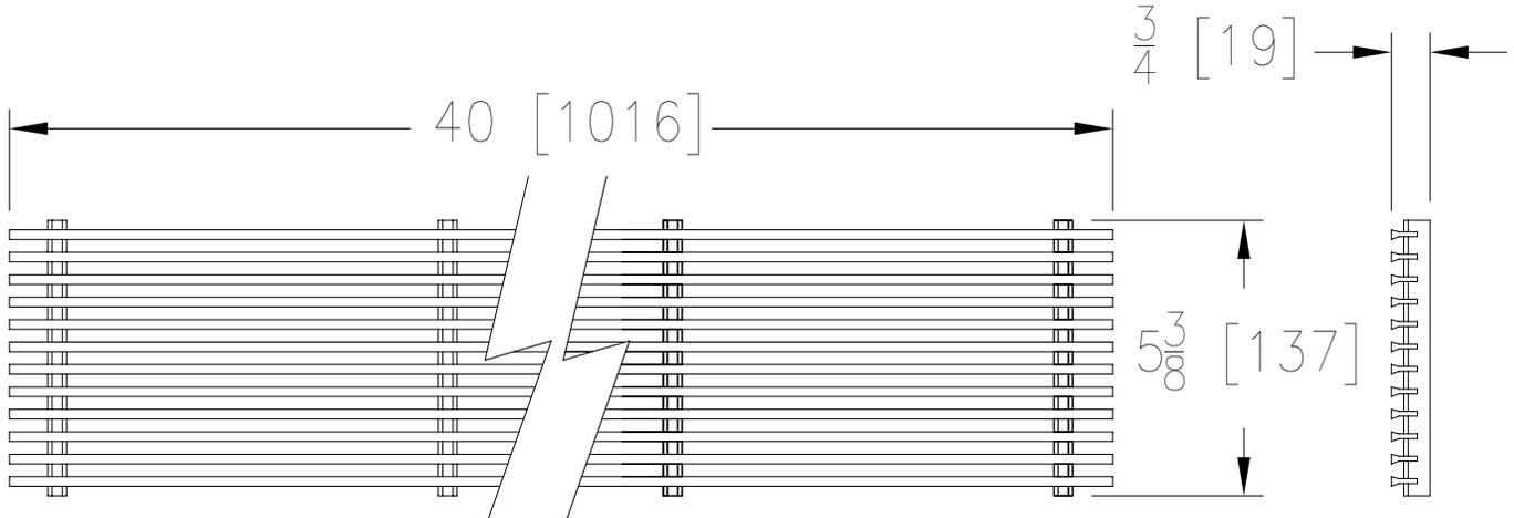
**AWG GRATE ENGINEERING SPECIFICATION: ZURN P6-AWG**
