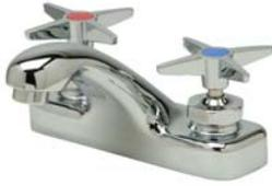
Polished chrome-plated cast brass faucet body with integral shanks, quarter turn ceramic disc cartridges and a 4" [102mm] long integral cast spout. Unit is furnished with a 2.2 GPM [8.3 L] pressure compensating aerator (complying with ANSI A112.18.1 Standard for flow), vandal-resistant color-coded metal four arm handles, mounting hardware and 1/2" NPSM coupling nuts for standard lavatory risers.
