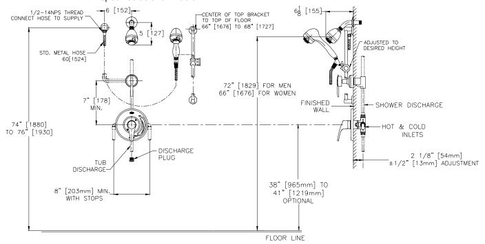
Note: All dimensions are for reference only. Do not use for pre-plumbing. Parts shown as hidden lines are supplied by others.
