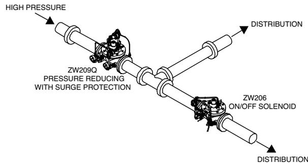
**Caution:** The recommended installation orientation for ACVs is horizontal, with the valve cover up. 6" and larger valves should only be installed horizontally, with the valve cover up, due to the difficulty of properly bleeding air out of the cover and performing maintenance on valves installed in the vertical orientation.
