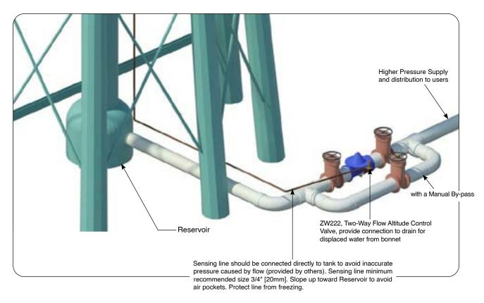
**Caution:** The recommended installation orientation for ACVs is horizontal, with the valve cover up. 6" and larger valves should only be installed horizontally, with the valve cover up, due to the difficulty of properly bleeding air out of the cover and performing maintenance on valves installed in the vertical orientation.
