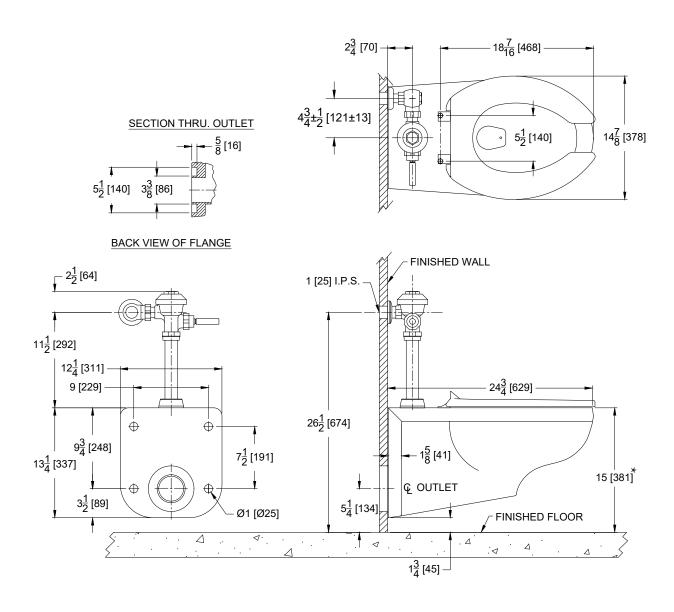
\*NOTE: For ADA compliance, top of seat height should be installed at 17" [431mm] -19" [482mm] from finished floor.
