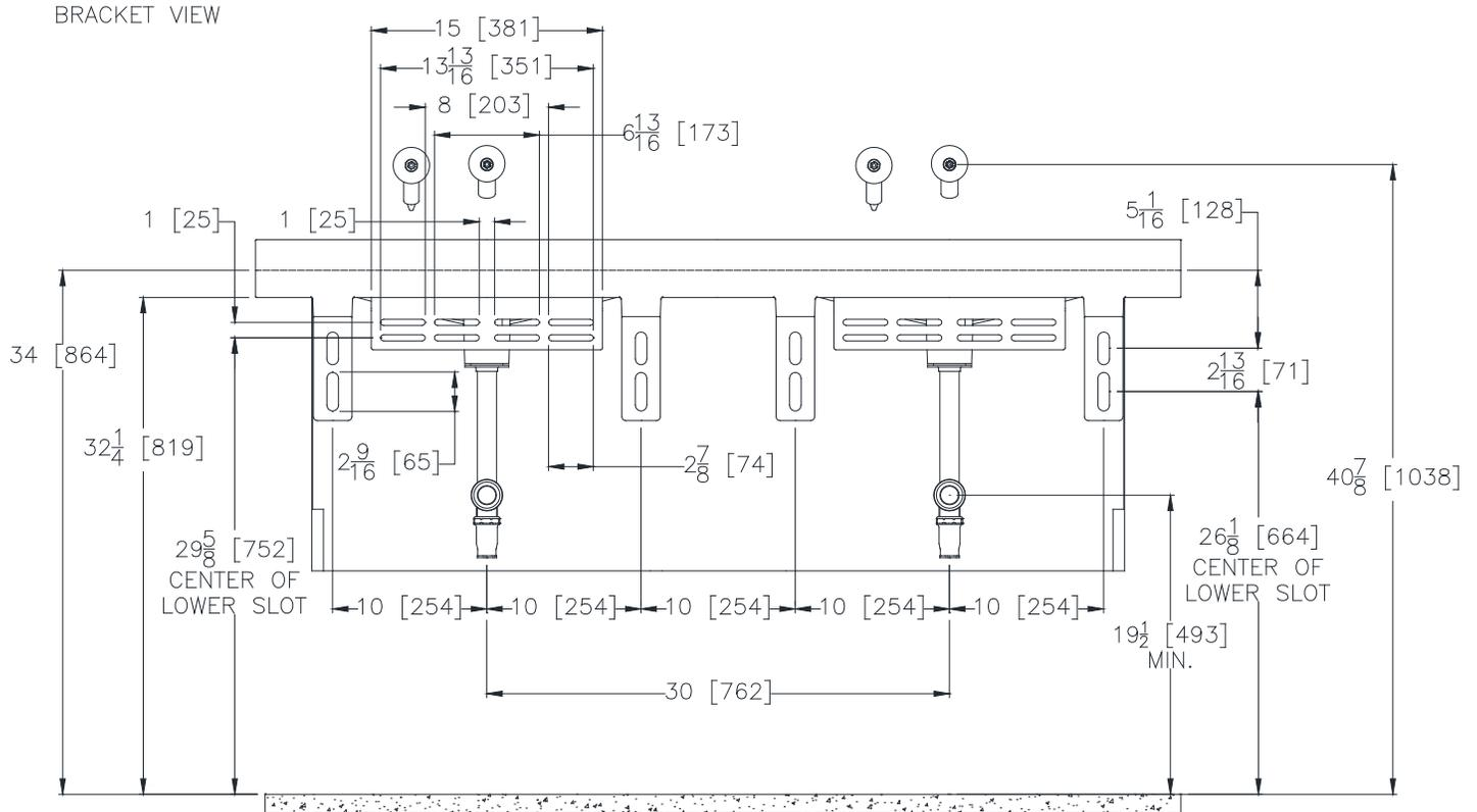
Installing the P-trap outlet lower than 19.5" from the finished floor will prevent the vandal shroud from being installed.
