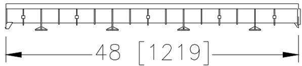
**ENGINEERING SPECIFICATION:** Zurn Z880 2 1/2 [64] Wide Trench Drain System shall be 48 [1220] long and 2 1/2 [63.5] wide. Drain shall be 3 [76] deep. Drain shall be made of (HDPE) High Density Polyethylene, and is UV-10 stabilized. Drain shall have bedding feet to be used for positioning and anchoring purposes. Drain shall have tongue and groove snap fit connection. Drain shall have 24 [610] long high-density polyethylene decorative grate (-POG) provided as standard.
