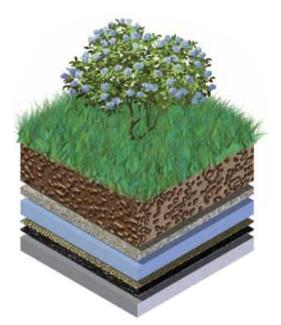
Z110 Green Roof Drain shown with 18" height for intensive green roofing applications. Z110 green roof drains are available with enclosure heights ranging from 5" to 18" or as specified.
