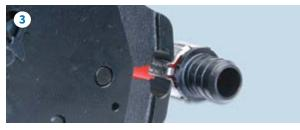
Using QickClamp tool, crimp the QickClamp pinch ear. (QCRTQCM shown)
