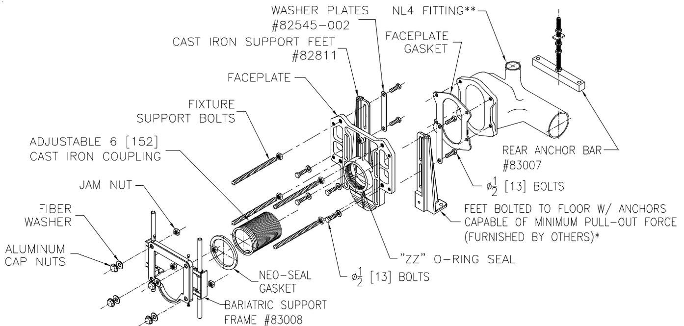
\*Carrier foot anchors must be able to withstand a pull-out force of 335 Lb.[152 kg.]. Calculated value, no safety factor applied.
