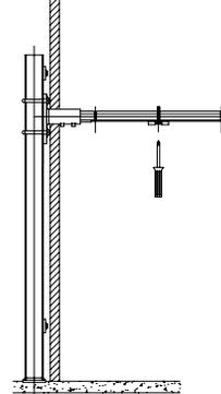
**3.** Gently slide lavatory onto the carrier arms to within 1/16" of the finished wall. The access holes on the underside of the lavatory should line up with the lockdown bar & adjustment screw holes of the arms.
