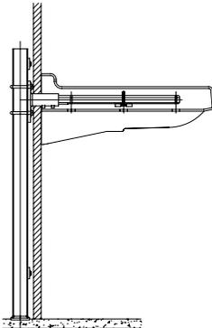
**4.** To make adjustments to the height and level of the lavatory, install the remaining (4) leveling screws by threading each screw up through the underside of the lavatory into the carrier arms, raising or lowering the fixture as necessary.
