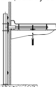
**6.** Caulk/Silicone lavatory to the finished wall for a water tight seal.
