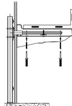
**5.** Once the lavatory is set to the proper height and leveled, gradually reverse the lock-down bar screw from the arm until the rubber pads of the lock-down make contact with the fixture, securely locking it into place.
