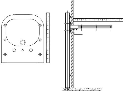
**2.** Install lavatory lock-down bar to arm by threading it up through the underside of the arm as shown, keeping the wings of the lock-down in line with the arm.
