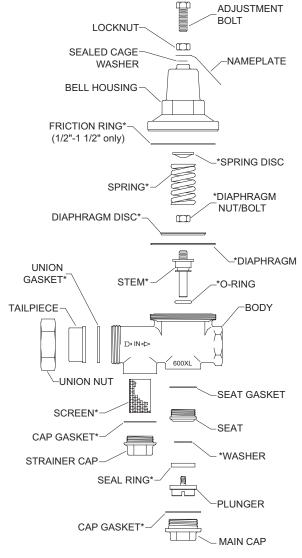
\* INDICATES PARTS SUPPLIED IN REPAIR KITS (spring disc not included in sizes 1 1/2"-2")
